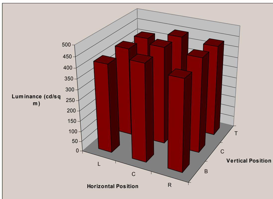
The AAPM TG18 Display Assessment protocol states that the maximum luminance variation should be less than 30%, this luminance variation being calculated by the formula  $L_{var} = 200 * (L_{max} - L_{min}) / (L_{max} + L_{min})$ .
