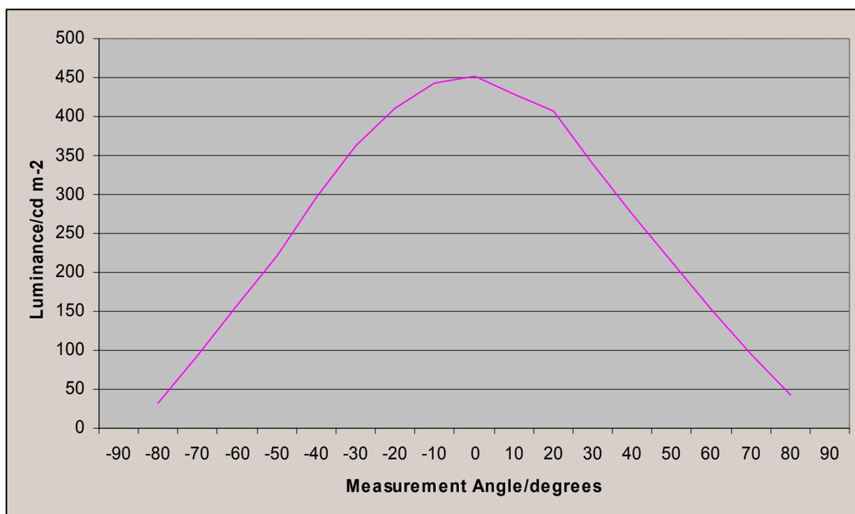
Figure 8 shows the variation of peak luminance as viewing angle varies vertically, with the display in portrait mode.
