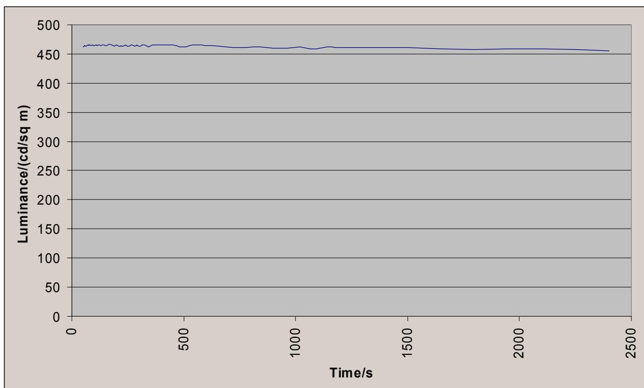
It can be seen that over the measurement period there was no significant drift in the peak luminance value measured.
