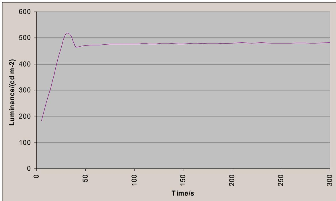
It can be seen that the device reached its target luminance and remained there after approximately one minute. In normal use, this would be well within the time required to start up the base PC and for the user to log in.
