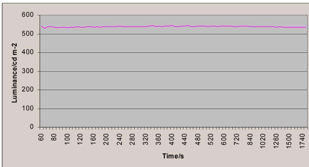
It can be seen that over the measurement period there was no significant drift in the peak luminance value measured.
