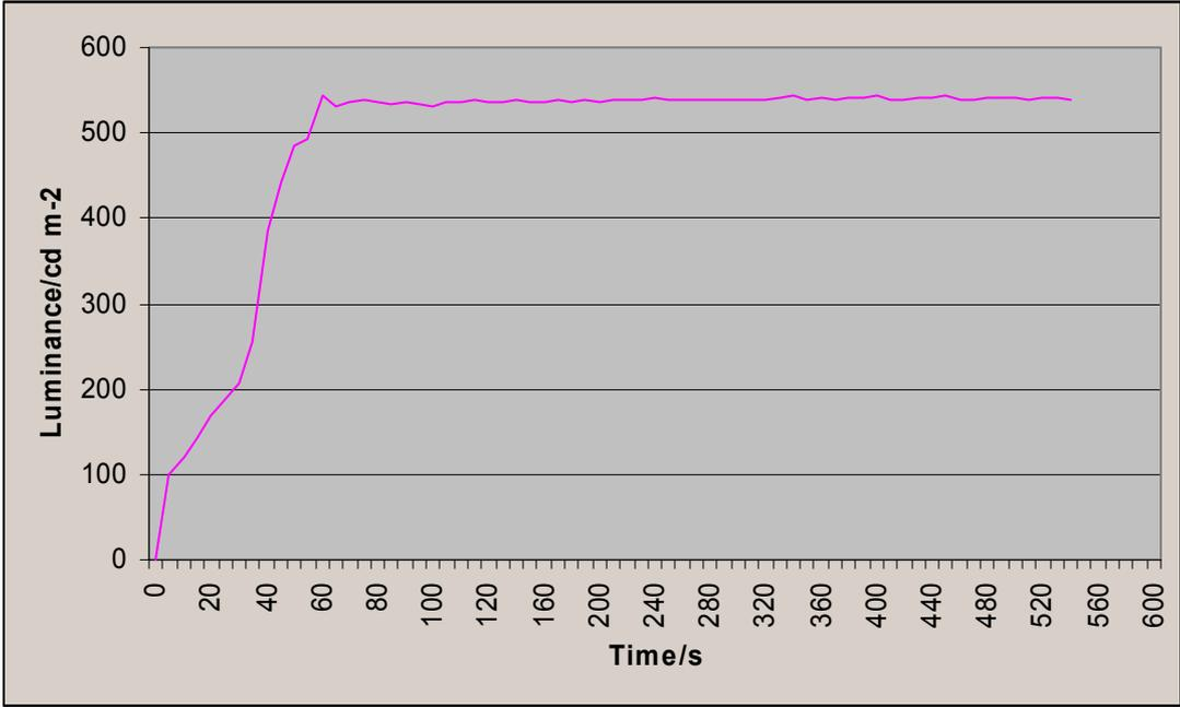
It can be seen that the device reached its target luminance after approximately one minute. In normal use, this would be well within the time required to start up the base PC and for the user to log in.
