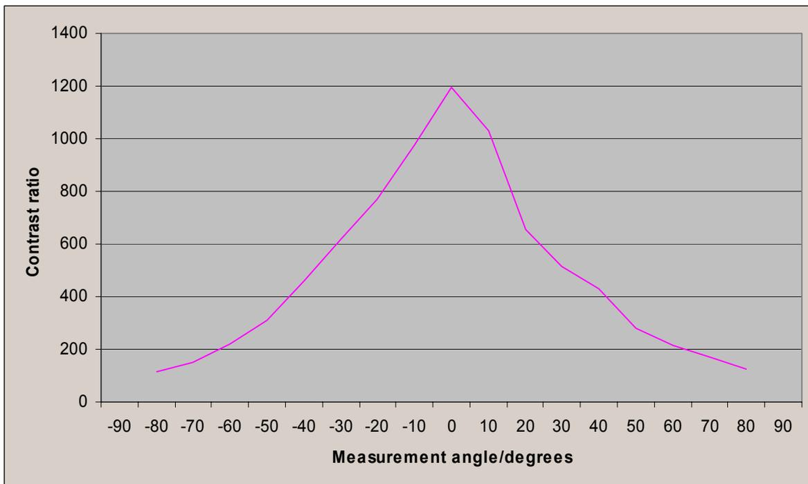
Figure 10. Variation of contrast ratio with viewing angle - vertical
