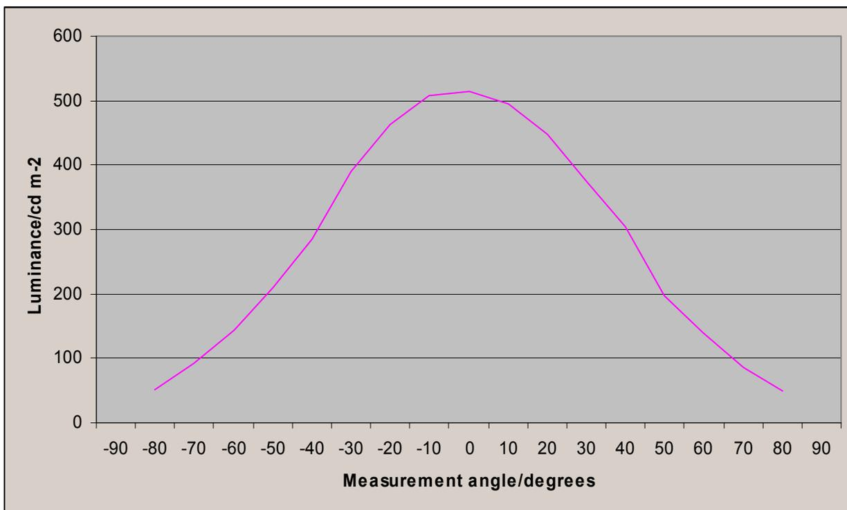
Figure 8. Variation of luminance ratio with viewing angle - vertical
